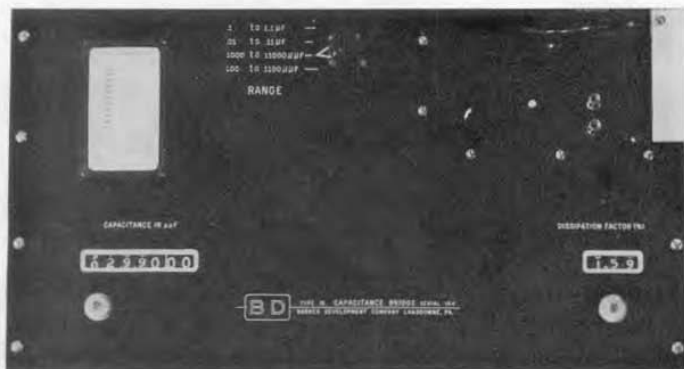
Figure 1. Panel view of the Barnes Automatic-Balancing Capacitance Bridge.
